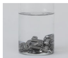
① Dip sample into solvent to extract oil
