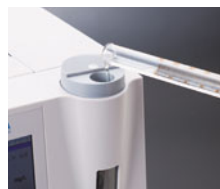
① Inject water sample, solvent
