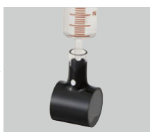
② Inject measuring solvent into cell
